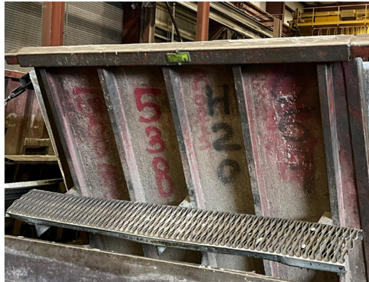
An example of an Idencia RFID tag on a mold at Shea Concrete.
