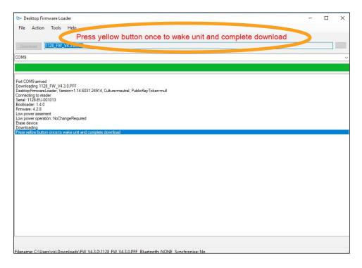
When prompted (see screenshot above) press the trigger button on the reader to wake the unit and complete the download.
